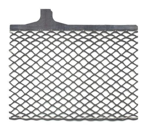
PRODUCED ON ROCHE EXPANDER 5 TOOTH (4 CUT, 1 REFORM)
