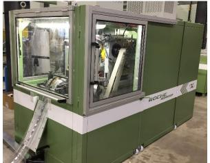
The machine is designed according to a double arch type with double crankshaft and direct drive. The frame is composed of a welded steel lower base and an upper arch fitted onto the base. The lower part receives the expanding tool and the power drive mounted on an adjustable base.
