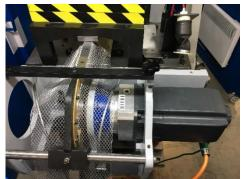
The pitch of the grid is easily adjustable through the HMI. That solution ease the setting of the line during tooling changeover.
