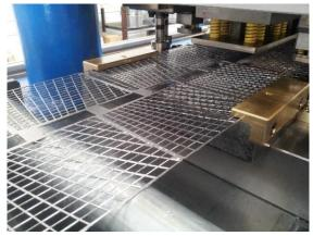
In case of different plate design, the tooling is easily exchangeable as all the needed equipment are already implemented into the PUNCHMASTER (hydraulic clamping, rollers and console).
