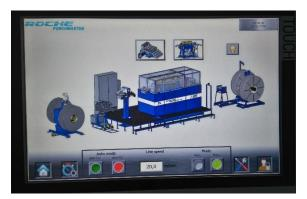
The whole synchronization of the line is done through ultrasonic sensors between each machinery.
