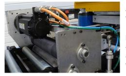
A specific strip feeding system has been developed specially for the PUNCHMASTER. It consists of 2 servo-motors with rollers located at the inlet and at the outlet of the tooling performing a push-pull feeding of the press. Low inertia rollers and a high performance brushless servo-motors provide a very accurate position of the strip between each stroke. The strip feeder synchronisation with the press is made with a cam.
